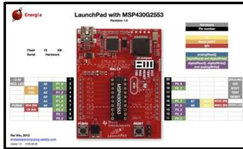
Figura 16. Diagrama LaunchPad Msp430g2553
